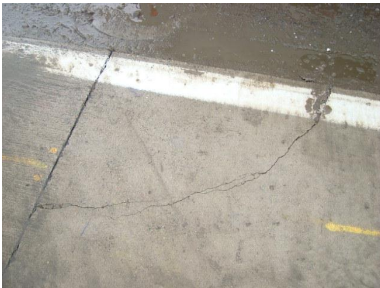
Figure 4-28. New Corner Break on Cell 32 during Spring 2010 Testing
