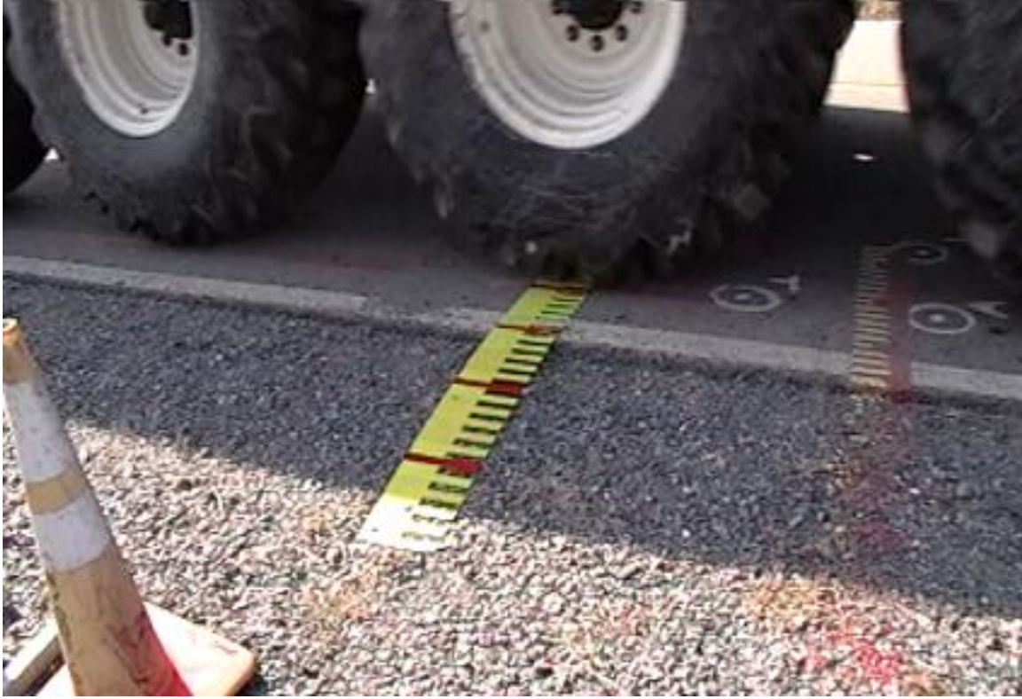
Figure 3-9. Illustration of Steel Scale Placement for Determination of Traffic Wander
