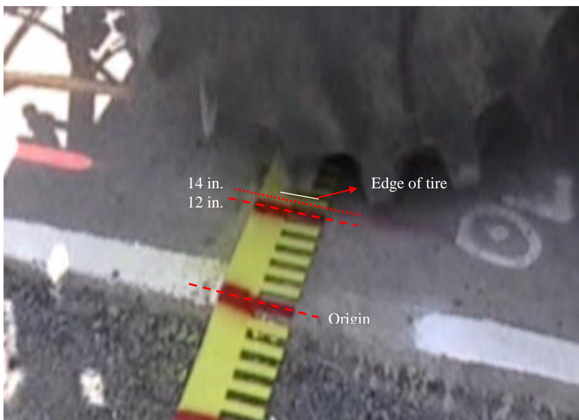
Figure 4-1. Determination of Vehicle Wheel Edge Offset
