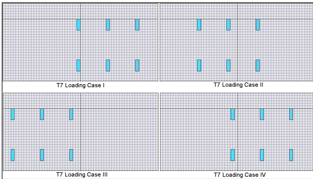
Figure 5-30. Loading Scenarios for T7 on 15 Feet Slab
